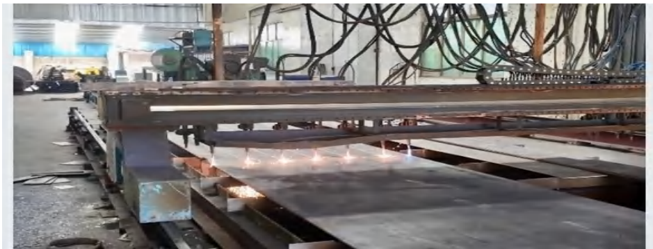
FLAME CUTTING - HEAVY PLATE GEOMETRY CHECK
